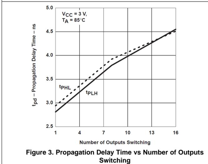
Figure 3. Propagation Delay Time vs Number of Outputs Switching
