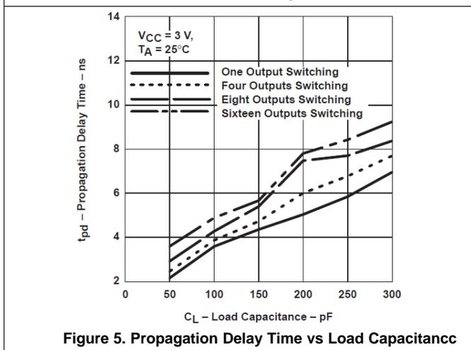
Figure 5. Propagation Delay Time vs Load Capacitance
