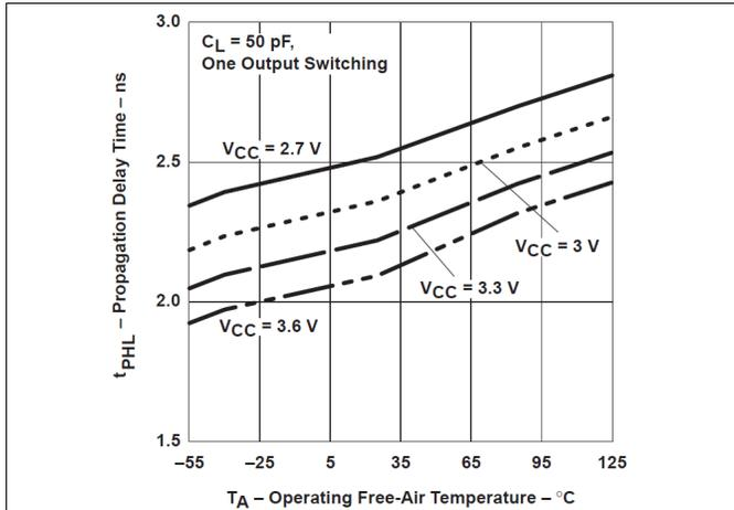
Figure 1. Propagation Delay Time vs Operating Free-Air Temperature
