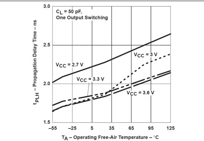
Figure 2. Propagation Delay Time vs Operating Free-Air Temperature
