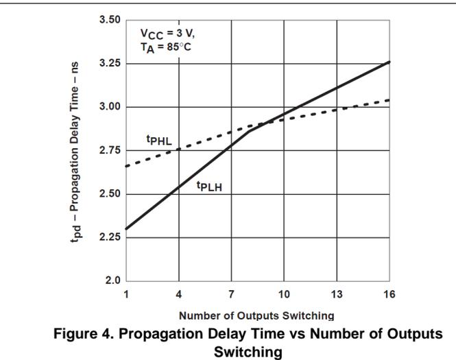
Figure 4. Propagation Delay Time vs Number of Outputs Switching
