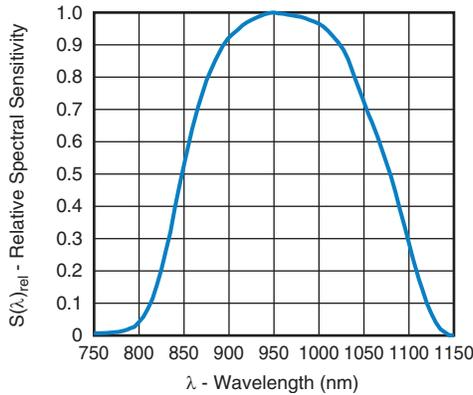
Fig. 8 - Relative Spectral Sensitivity vs. Wavelength
