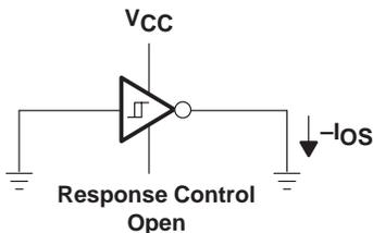
NOTE A: Arrows indicate actual direction of current flow. Current into a terminal is a positive value.
