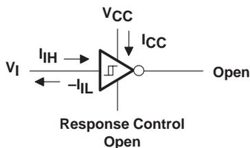
NOTE A: Arrows indicate actual direction of current flow. Current into a terminal is a positive value.
