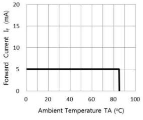
Fig. 2 FORWARD CURRENT VS. DERATING CURVE
