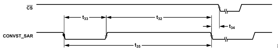
Figure 5. SAR ADC Timing Diagram
