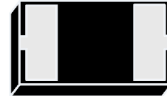
DFN1006-2L (Bottom View)
